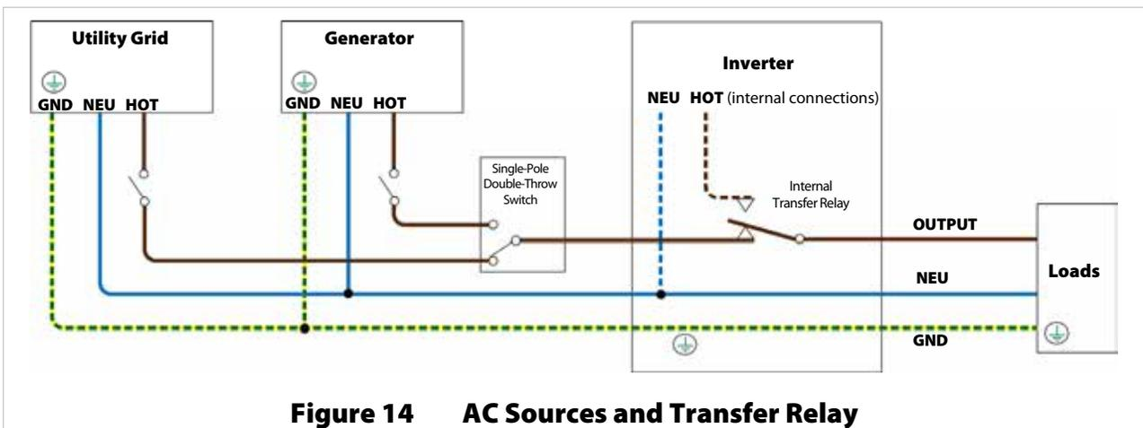
**Figure 14 AC Sources and Transfer Relay**
