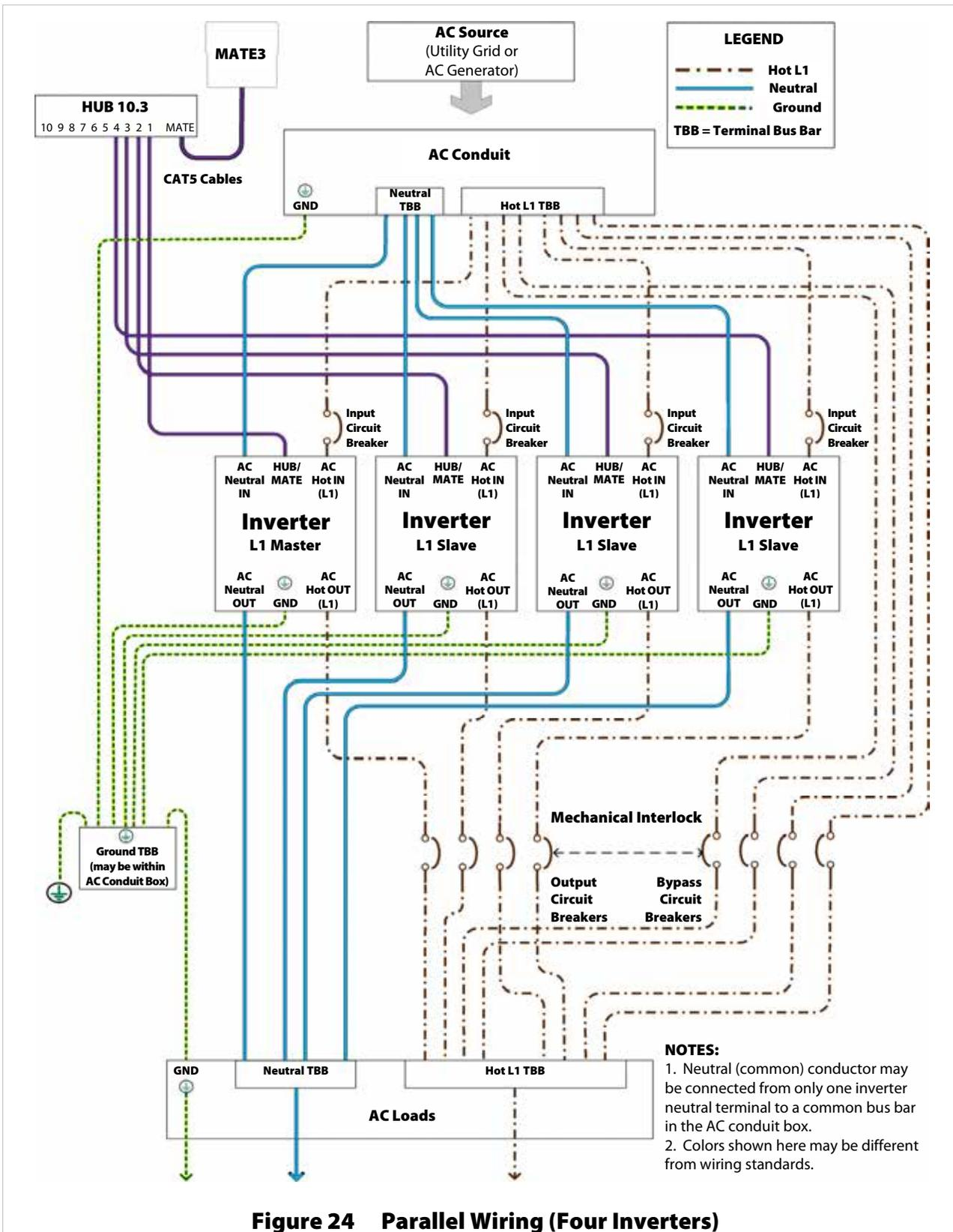
**Figure 24 Parallel Wiring (Four Inverters)**
