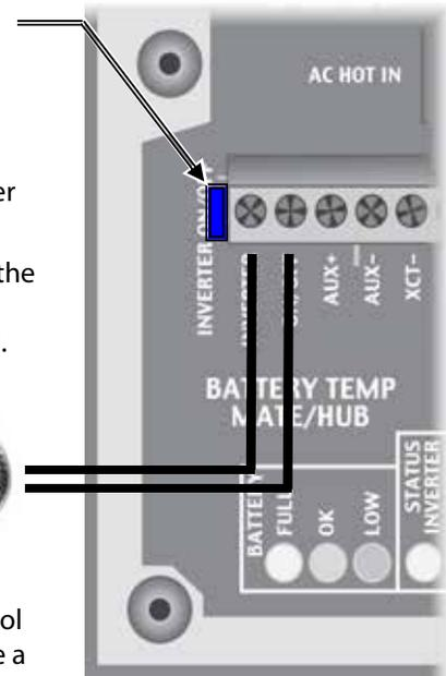
**Figure 15 ON/OFF Jumper and Connections**
