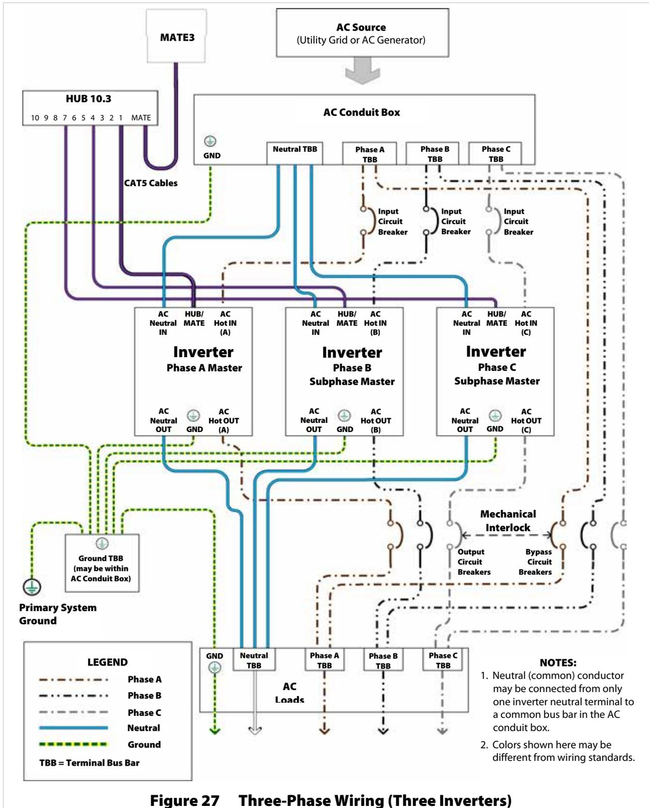
**Figure 27 Three-Phase Wiring (Three Inverters)**
