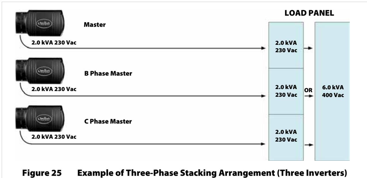
**Figure 25 Example of Three-Phase Stacking Arrangement (Three Inverters)**
