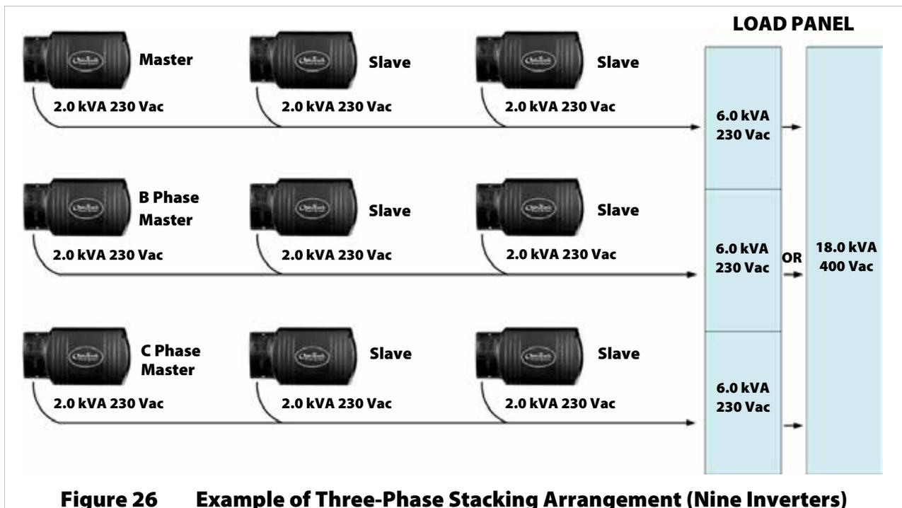
**Figure 26 Example of Three-Phase Stacking Arrangement (Nine Inverters)**
