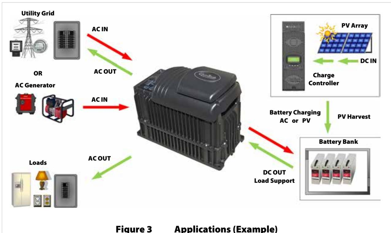
In Figure 3, the inverter uses a bidirectional AC input to sell power back to the utility grid. The power being delivered to the grid (labeled "AC Out") is excess AC power not being used by the AC loads. Selling requires an inverter/charger with **Grid Tied** mode available and active.
