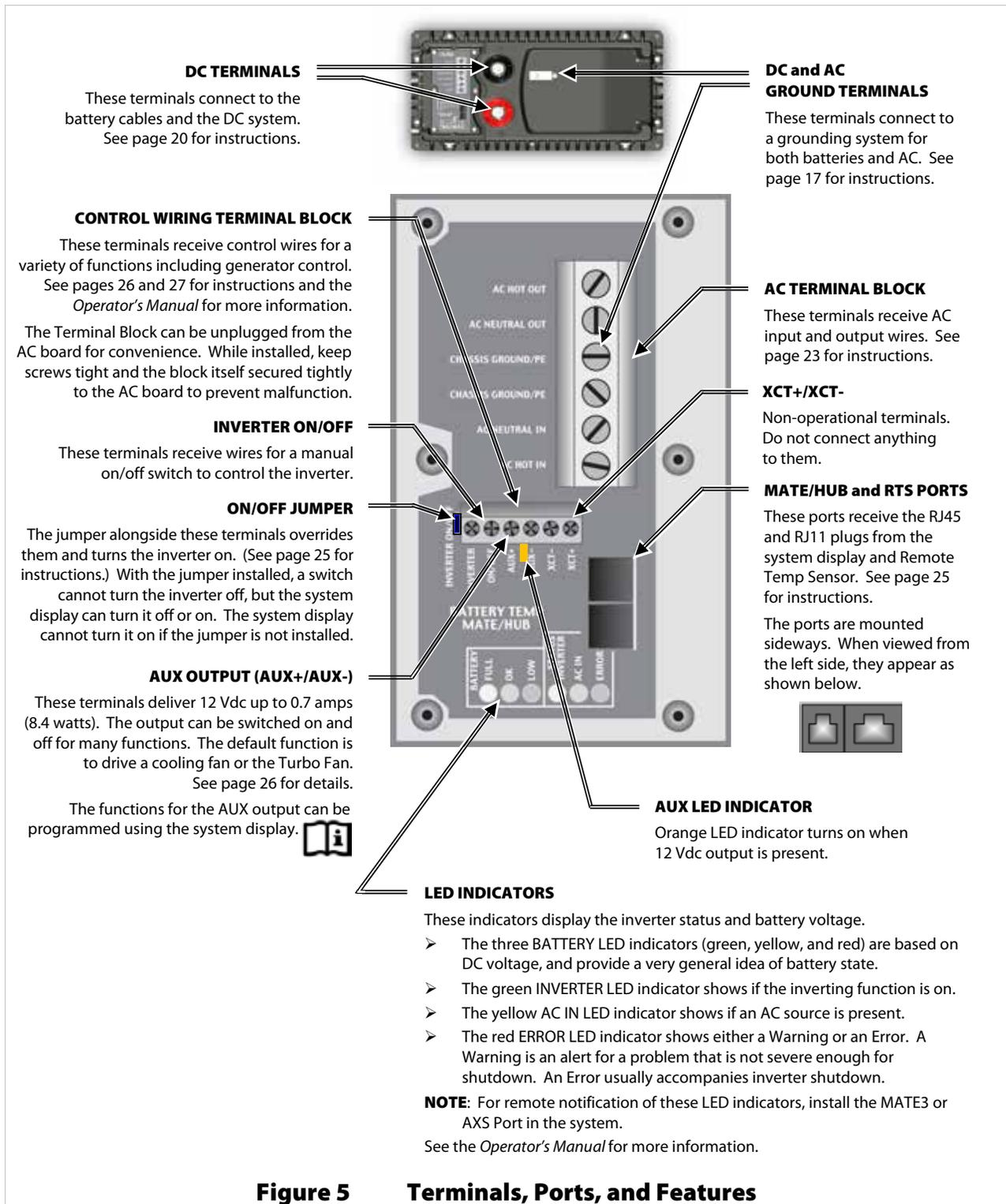
**Figure 5 Terminals, Ports, and Features**
