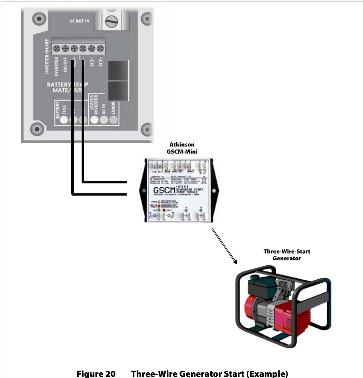
**Figure 20 Three-Wire Generator Start (Example)**
