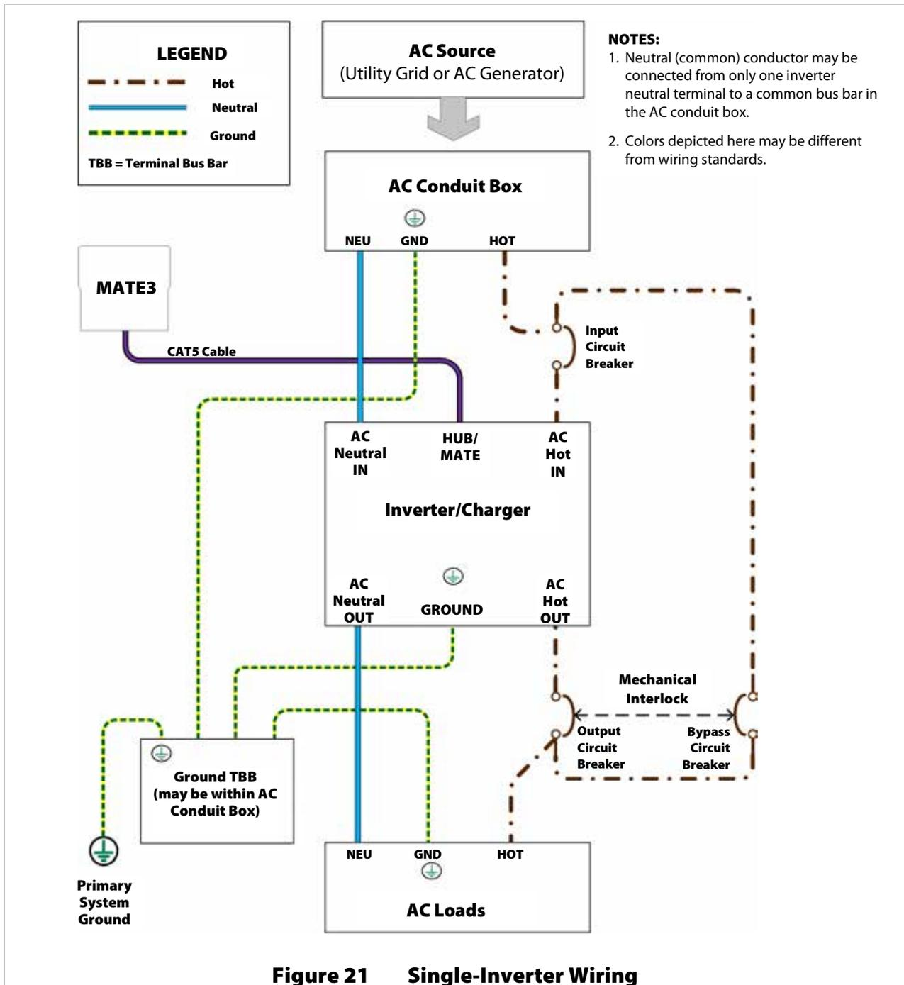
Figure 21 Single-Inverter Wiring
