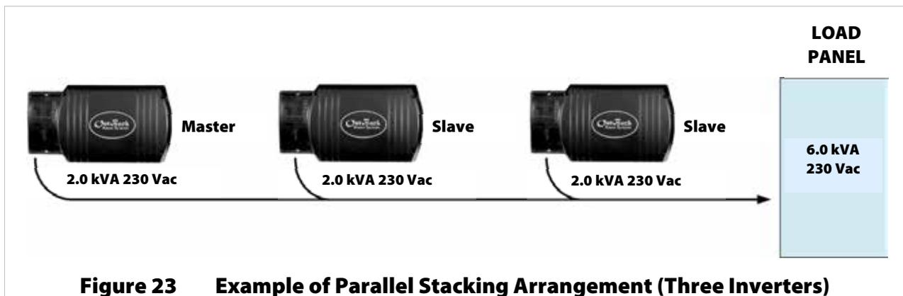
**Figure 23 Example of Parallel Stacking Arrangement (Three Inverters)**
